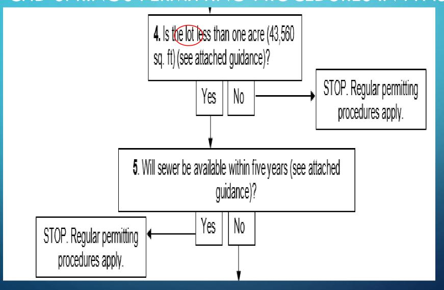
**6**. Inform applicant a nitrogen-reducing system is required. The applicant has the following options: choose an NSF245-certified aerobic treatment unit (ATU) or choose a nitrogen-reducing performance-based treatment system (PBTS). Once rulemaking is finalized, the applicant may be able to choose an in-ground nitrogen reducing biofilter (INRB), but this is not currently an option.
